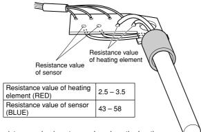
If the resistance value is not normal, replace the heating element.
