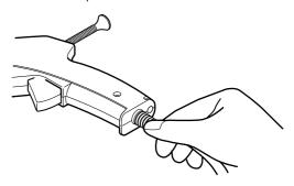
Check the resistance value between the pin of the plug and the wire on the terminal.
